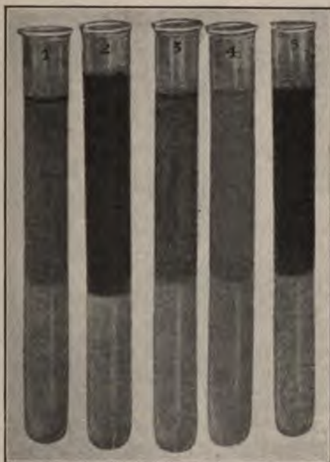
FIG. 45.—Diffusion of colloids into 2 per cent. agar-agar at the end of a week. 1, Gold hydrosol; 2, silver solution ( Credé ); 3, antimony sulphide solution; 4, arsenic trisulphide solution; 5, iron hydroxide solution.
